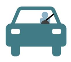
The purpose of the seatbelt is to help prevent injuries and fatalities resulting from colliding with objects or people in the vehicle, and to prevent ejection from the vehicle in the case of a collision.
